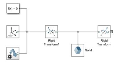
In the Solid block dialog box, specify the following parameters. Later, you define the MATLAB variables shown using a Subsystem block that contains the Solid and Rigid Transform blocks. Among its advantages, this approach enables you to update variables used in multiple blocks from a single place—the Subsystem block dialog box.
