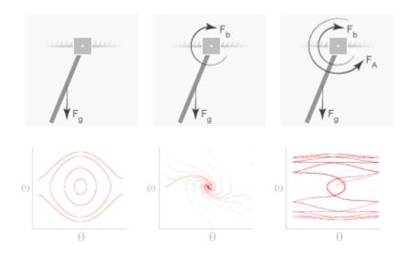
Your starting point is the simple pendulum model that you built in "Model a Simple Pendulum" on page 1-16. By adding forces and torques to this model, you incrementally
