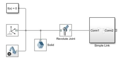
In the Solid block dialog box, specify the following parameters. This block connects rigidly to the World frame and therefore has no effect on model dynamics. You can leave the inertia parameters in their default values.
