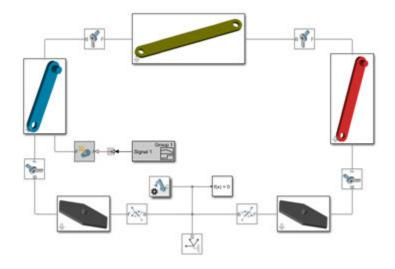
To specify the force or torque acting at a joint, Simscape Multibody provides a selection of actuation inputs directly in the joint blocks. Each joint primitive—the basic component of a joint block—provides a selection of actuation inputs specific to that primitive.
